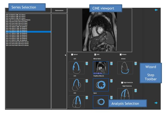
QStrain reads both MR and CT data. It allows 4 different types of analysis: Apical (LAX), SAX, Atrium and Right Ventricle. Each slice can be assigned to its appropriate block depending on the orientation and the analysis to be performed.
